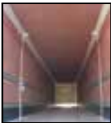
Optional heated box with interior plywood lining.
